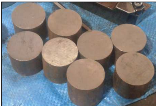
Figure 1: 080M40 steel Sample bars
